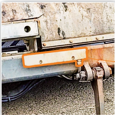
■ Example of RFID antenna installation for Frontloader vehicles
