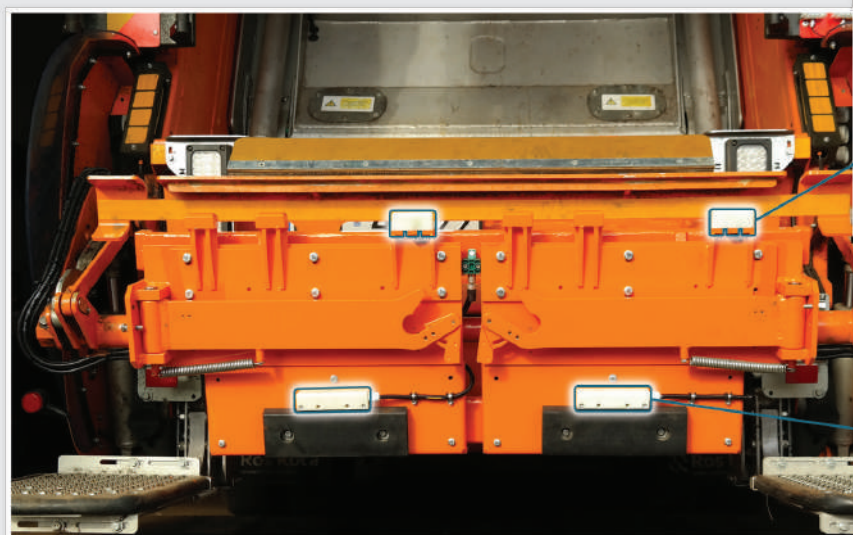
■ Example of RFID antenna mounting on a vehicle with rear loading
